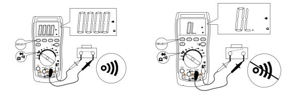
D) Connect the test lead to the two ends of tested circuit in parallel. E) If the value of resistance between the two ends of the tested circuit is less than  $(70\pm30)\Omega$ , buzzer inside sounds.
