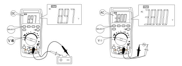
B) Insert the red and black test lead separately to  $V\Omega\,\text{Hz}$  and COM input terminal.
