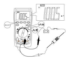
B) Insert the red and black test lead separately to uAmA and COM input terminal.
