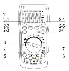
4. 10A current input terminal: Measuring AC/DC 10A positive input terminal, insert the red test lead.
